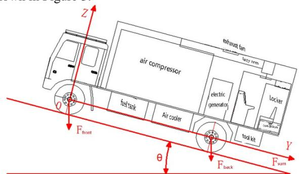
Figure 3: Maneuvering rescue platforms longitudinal stability diagram.
