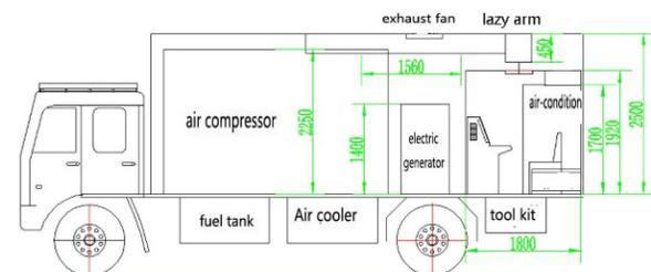
Figure 1: Layout left view of the maneuvering rescue platforms.
