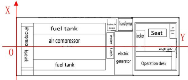
Figure 2: Maneuvering rescue platform x-y coordinate system schematic.
