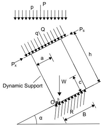
Figure 1: The hydraulic support mechanic model of anti-dumping along face dip.
