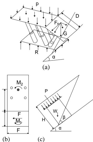
Figure 4: The anti-rotation mechanic model of support tail beam.
