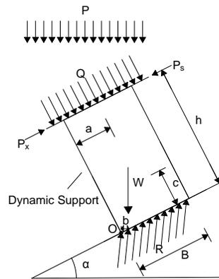
Figure 3: The simplified hydraulic support mechanic model of anti-slip along face dip.
