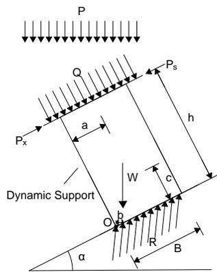
Figure 2: The simplified hydraulic support mechanic model of anti-dumping along face dip.
