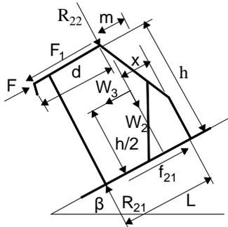
Figure 5: The support mechanic model of anti-dumping along strike when downhill-mining.
