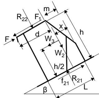
Figure 6: The support mechanic model of anti-slip along strike when downhill-mining.
