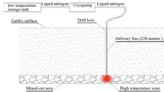
Figure 6: Liquid nitrogen injection process.
