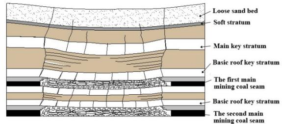
Figure 3: Schematic diagram of mining-induced fractures connected to the ground surface.
