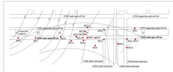
Figure 7: Location map of drill holes MH26–MH45 for liquid nitrogen injection.
