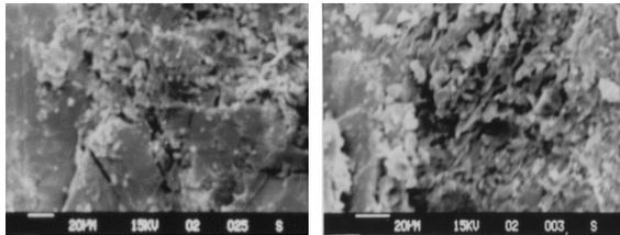
Figure 1: SEM image of pore structure of coal (a) before water soaking; (b) after water soaking.
