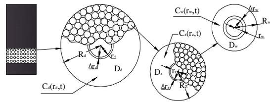
Figure 2: Conceptual model for tridisperse pore structure.
