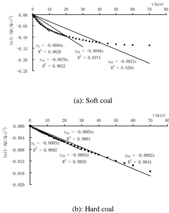
Figure 1: Fitting curves of Juji coal samples according to the unipore model.
