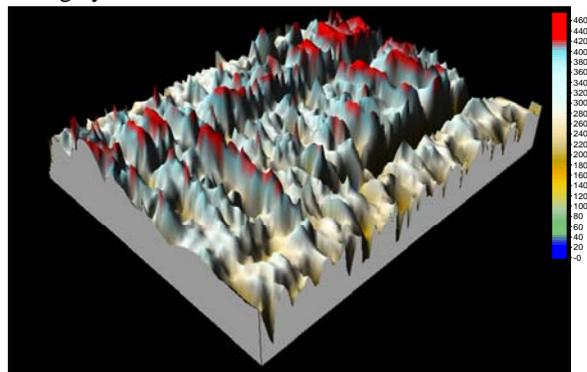
Figure 8: 3D map of the relationship among working face, shield pressure, and advancing distance.
