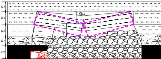
Figure 4: Schematic failure of lower sub key strata.
