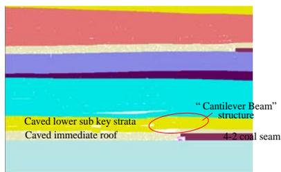
Figure 6: “Cantilever Beam” structure (270 m advancing).
