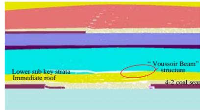
Figure 7: “Voussoir Beam” structure (230 m advancing).
