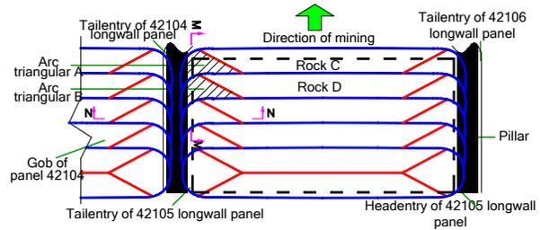
Figure 1: Schematic diagram of the broken form of the lower sub key strata.
