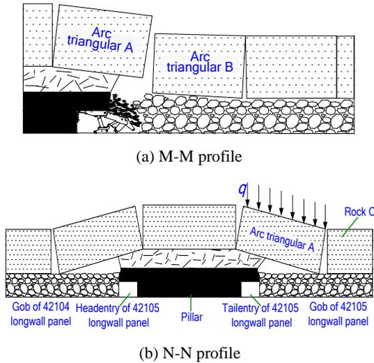
Figure 3: "Cantilever Beam" structure (thin immediate roof).
