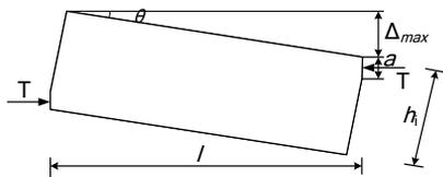
Figure 5: Limit equilibrium condition when the hinge contacts of rock blocks are in plastic state.
