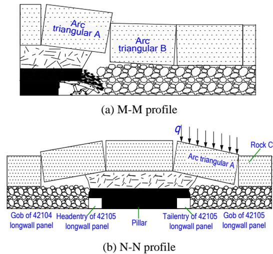
Figure 2: “Voussoir Beam” structure (thick immediate roof).
