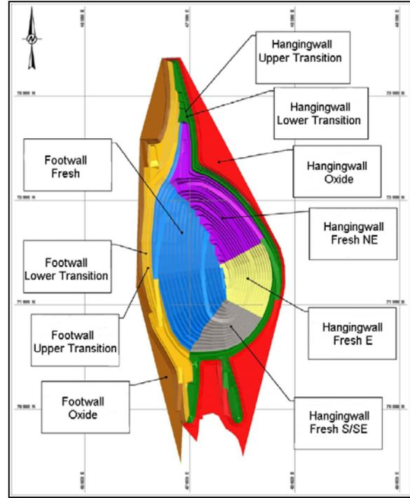
Figure 3: West Branch open pit geotechnical sectors. Modified from Golder (2014).
