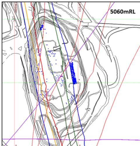
Figure 14: Plan view of West Branch major structure and wet drill hole mapping correlation.
