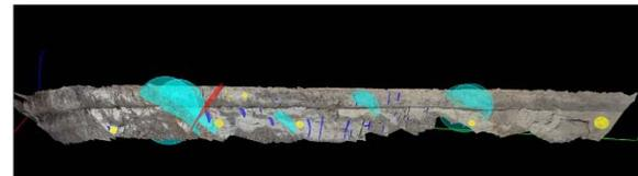
Figure 12: Structural measurements obtained along the West Branch footwall using photogrammetry.
