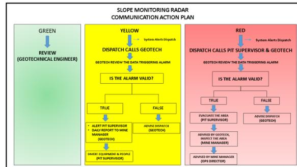
Figure 16: Summary of the slope movement action plan.
