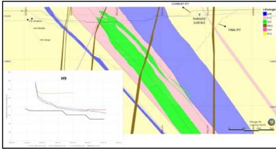
Figure 13: Cross section of vibrating wire piezometer hole.
