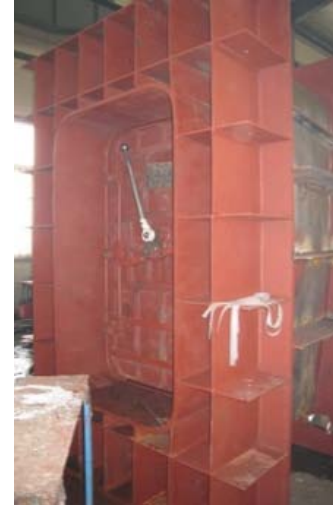
Figure 6: Protective door and sealed container for water proofing test.
