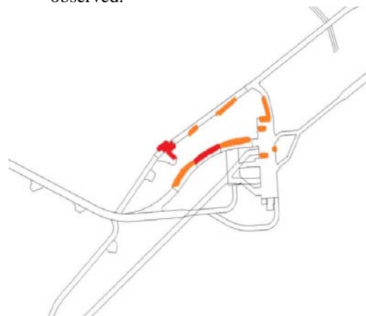
Figure 6: Rockbursts record in the Powerhouse area.
