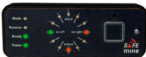
Figure 1: SAFEmine LED display showing vehicle locations and distances (e.g. green LED indicates a vehicle to the left at 100 m, red LEDs indicate vehicles behind and to the right at 50 m).
