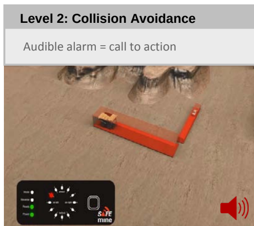
Figure 6: Collision avoidance function provides audible alarms and visual indicators when two vehicles are on a collision course as determined by their Dynamic Safety Zones.
