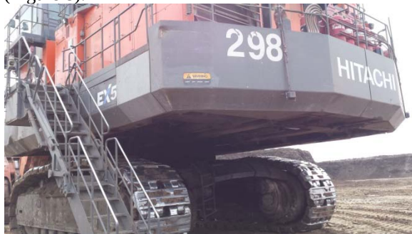
Figure 8: Rear mounting locations for TrackingRadar (just below counterweight).
