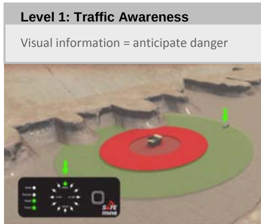
Figure 5: Traffic awareness function provides the operator with location and distance to nearby vehicles.
