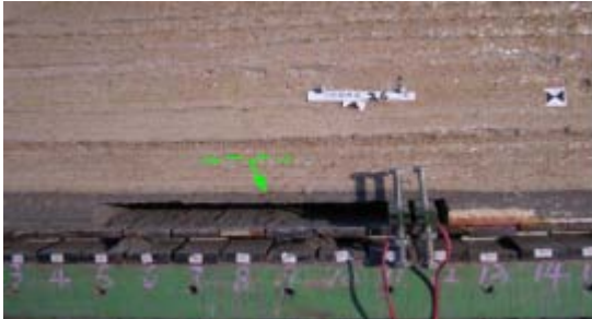
(a) Separation layer of coal roof (the working face is to 26 m)
