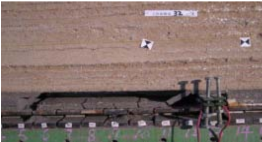
(b) Separation layer of coal roof (the working face is to 32 m)
