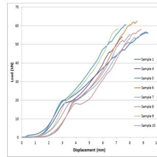
Figure 7: Single shear test results of 22 mm diameter dowels tested for single shear.
