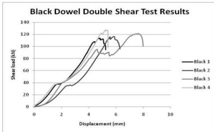
Figure 9: load displacement profiles of four double shear tests in steel frame.
