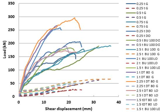
Figure 12- Shear pretention loads versus vertical displacement of double shear testing of 11 dowels.
