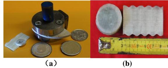
Figure 13a: Punch shear apparatus, Figure 13b: Punch shear apparatus.
