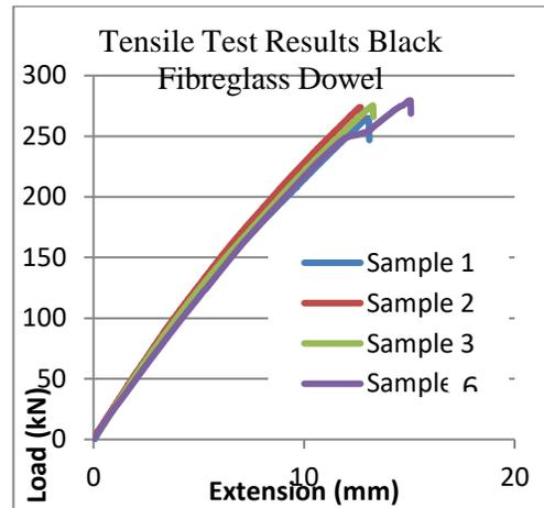
Figure 3: Load displacement profiles of four tested black dowel samples.
