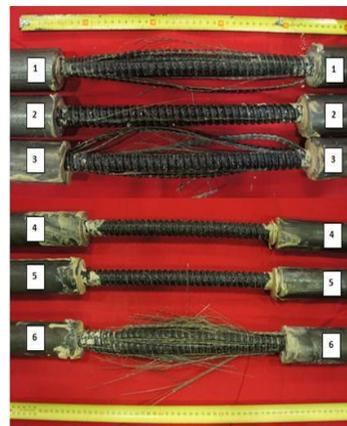
Figure 4: Tensile failure of four out of six tested samples.
