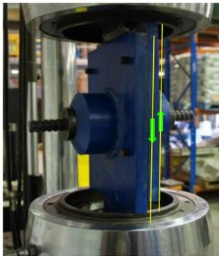
Figure 5: Single shear testing of black dowel.
