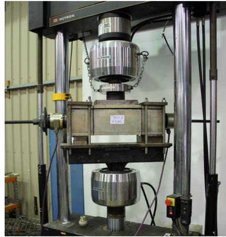
Figure 11: A double shear assembly mounted in the 500 kN Instron testing machine.
