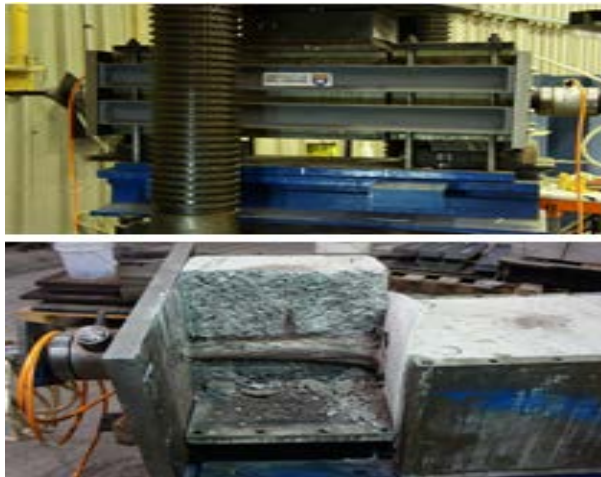
Figure 16: Up to date double shear instrument (a) the whole assembly inside compression machine (b) Teflon sheet layers between concrete blocks.
