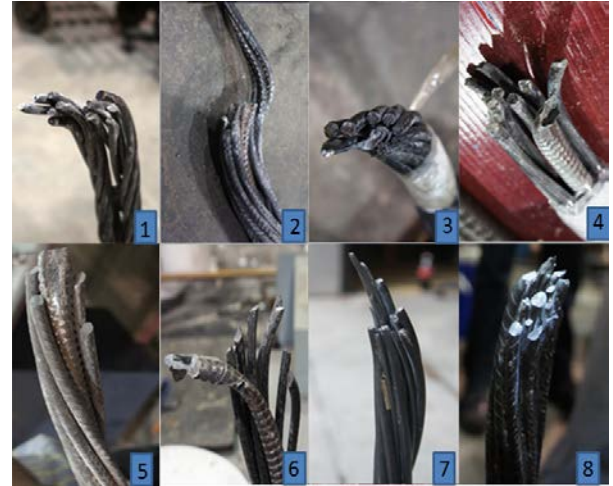
Figure 14: Strands snapped of the tested cables.
