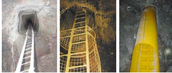
(a) Simple steel design (b) Steel cage (c) Laddertube Figure 1: The evolution of escapeway ladders.
