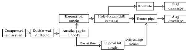
Figure 2: The mechanism of the underground reverse circulation sampling.
