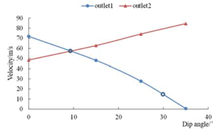
Figure 15: The flow velocity of outlet1 and outlet2 changed with the dip angle of the bit nozzle.
