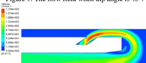
Figure 10: The flow field when dip angle is 55°.
