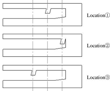
Figure 16: The bit nozzle models of different location.
