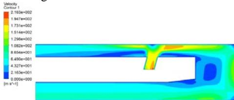
Figure 17: The velocity images when bit nozzle is in location ①.
