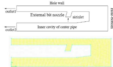
Figure 3: The simplified model and mesh of sampling bit.
