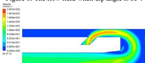
Figure 9: The flow field when dip angle is 45°.
