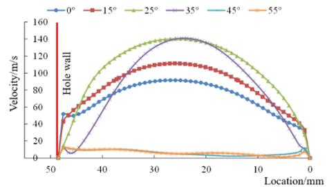
Figure 12: The velocity distribution of different location in the center cross section of the drilling cutter.
