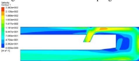
Figure 7: The flow field when dip angle is 25°.
