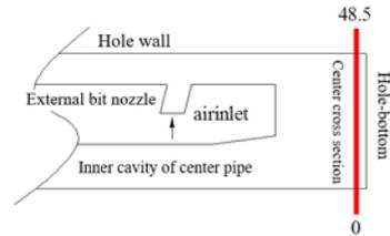
Figure 11: The location of center cross section of the drilling cutter.
