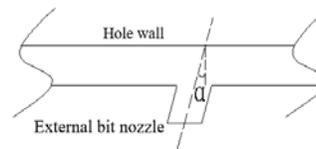
Figure 4: The dig angle of external bit nozzle.
