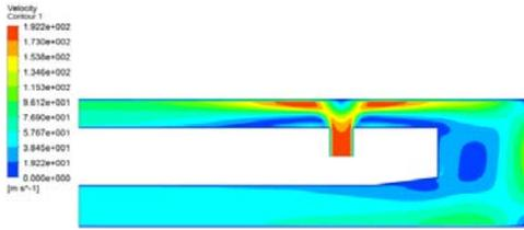
Figure 5: The flow field when dip angle is 0°.
