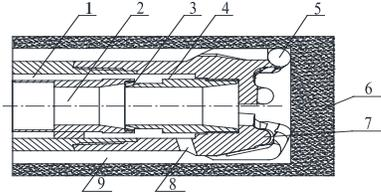
1-annular space, 2- center pipe, 3- jet nozzle, 4-annular ejector, 5- drilling cutter, 6-coal wall, 7- bit body, 8- external bit nozzle, 9- gap between the drill bit and hole wall
