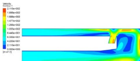
Figure 18: The velocity images when bit nozzle is in location ②.
