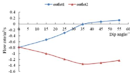
Figure 14: The flow rate of outlet1 and outlet2 changed with the dip angle of the external nozzle.
