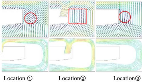
Figure 20: Velocity vector diagram and flow chart of bit nozzle in different position.
