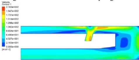
Figure 6: The flow field when dip angle is 15°.
