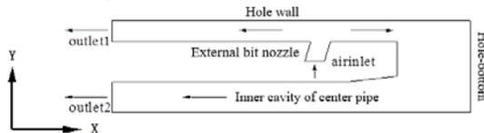
Figure 13: The flow direction in the model inner.
