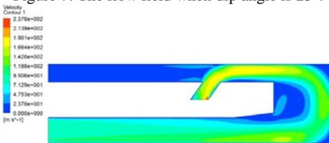
Figure 8: The flow field when dip angle is 35°.
