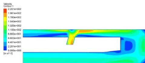
Figure 19: The velocity images when bit nozzle is in location ③.
