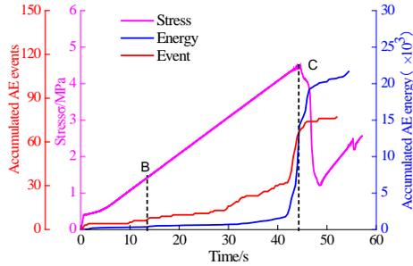
Figure 3: AE parameter variation of three slots sample with two level distributed.
