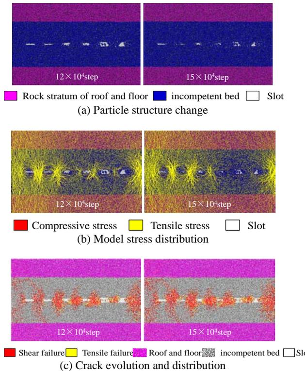
Figure 7: Crack evolution of single-level slots model in loading.
