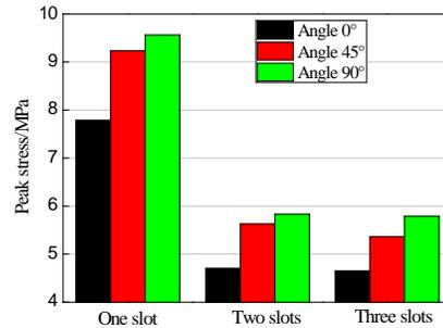
Figure 2: Peak stress distributions of different slotted samples.
