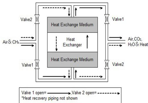
Figure 1: Schematic of two-bed type TFRR.
