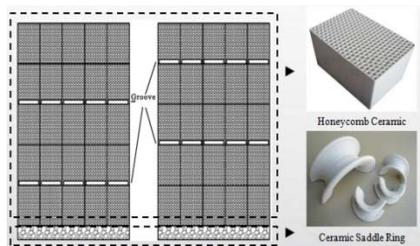
Figure 5: Schematic diagram of ceramic's layout.
