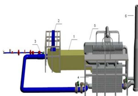
1. Diffusing tower. 2. VAM collecting cover. 3. Mixer. 4. TFRR. 5. Waste heat boiler. 6. Chimney.
