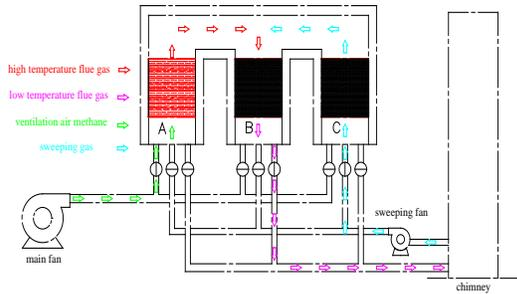
Figure 3: Structure schematic diagram of three-bed type TFRR.
