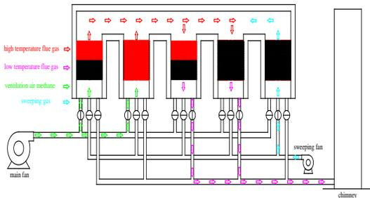
Figure 4: Structure schematic diagram of five-bed type TFRR.
