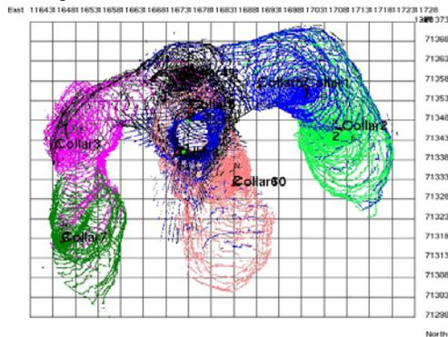
Figure 5: Anjialing goaf three-dimensional laser scanning the overall situation point cloud (Overlook).
