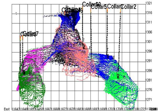
Figure 6: Anjialing goaf three-dimensional laser scanning the overall situation point cloud (Front view).
