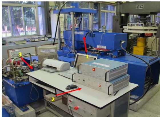
Figure 5: Large scale direct shear testing machine.
