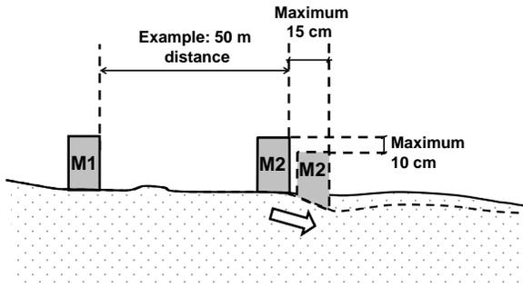
Figure 2: The environmental criterion for allowable mining-induced ground deformations, illustrated for a hub-to-hub distance of 50 m.
