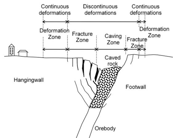
Figure 1: Mine-induced fracturing and deformations on the hangingwall and footwall in sublevel cave mining (schematic, not to scale).
