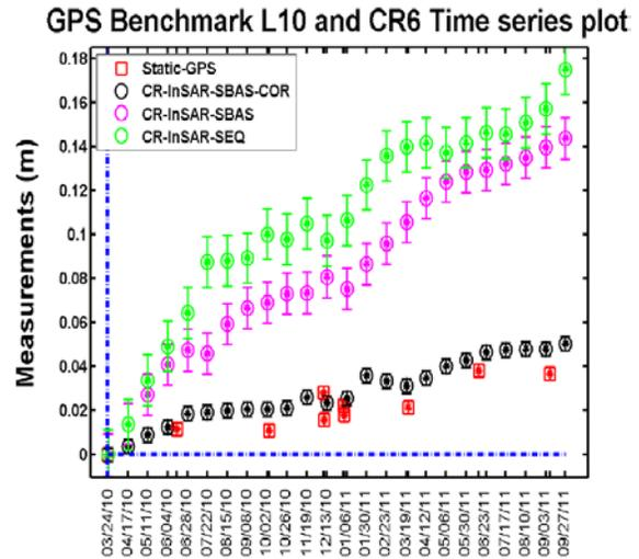
Figure 6: Time series plots of double difference CRInSAR measurements (CR6) and double difference Static-GPS measurements (L10) for different InSAR analysis techniques.
