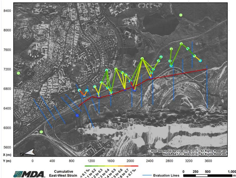
Figure 7: Spatial distribution of CR strain measurements in the east-west direction for the period of March 2010 to April 2014, with green representing low strain and red representing high strain. The environmental criterion limit determined from GPS measurements, corresponding to 0.3 % strain, is shown with a red line.
