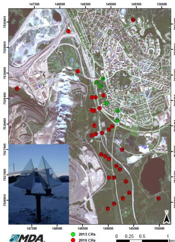
Figure 4: Corner reflectors (CR; see inset) installed in the Kiruna area.
