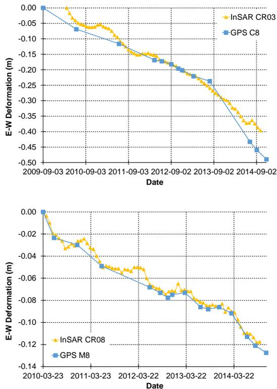
Figure 5: Cumulative deformation measurement for CR03 and CR08, compared with GPS data from nearby points C8 and M8, in the east-west direction.
