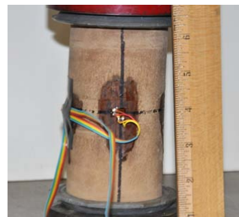
Figure 8: Paste backfill sample equipped with strain gauges.
