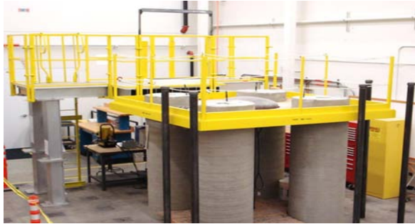
Figure 9: High-Energy High-Displacement test machine for conducting large-scale tests with reinforced shotcrete panels.
