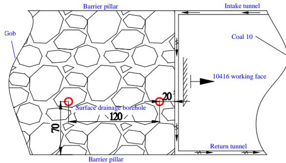
Figure 1: Tunnel arrangement of 10416 working face, Yangliu coal mine (units are in meters)
