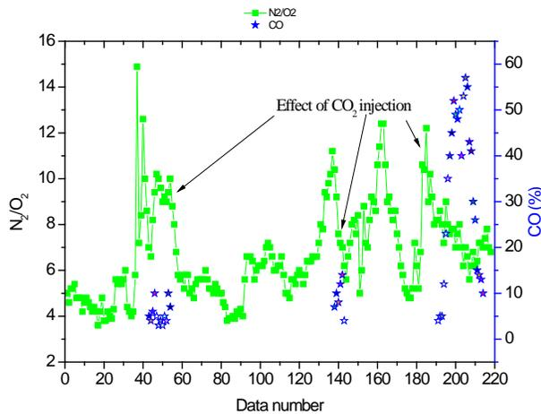
Figure 4: The variation of  $\text{N}_2/\text{O}_2$  ratio during methane draining from surface boreholes
