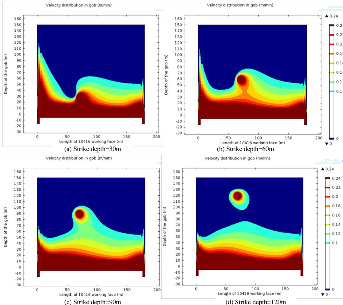
Figure 3: The influence of strike location of surface drainage borehole on spontaneous combustion in gob
