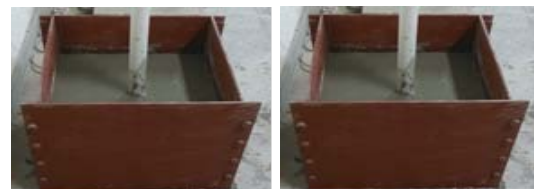
Figure 3. Pouring process of the secondary shotcrete lining, (a) before pouring, (b) after pouring.
