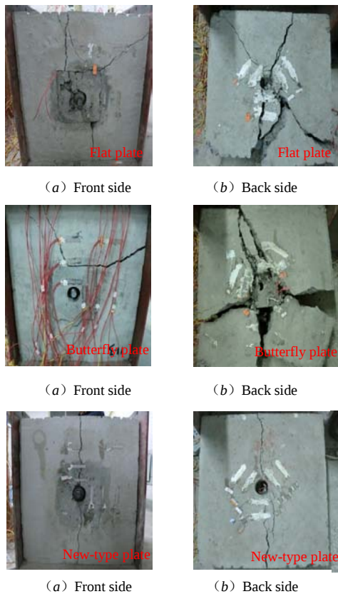
Figure 7. Fracture morphologies of C20 plain shotcrete linings
