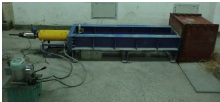
Fig.1. The self-developed multi-function bolt mechanical test system
